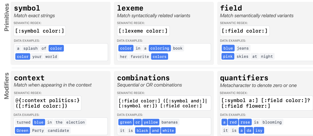
Figure 1: The semantic regex language consists of a set of primitives (top) that can be applied independently or combined with modifiers (bottom) to express diverse feature activation patterns.
