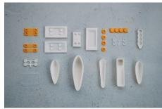
Figure 4: Molds and inserts for casting the silicone
