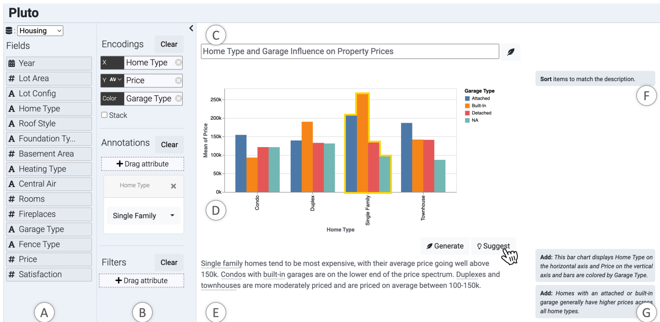
Figure 2: PLUTO’s user interface. The key components include a data panel (A), chart editor (B), chart title (C), main chart canvas (D), and a chart description (E). Here, the user has manually entered a description and clicked the Suggest button to get ideas on improving the chart and text for communication purposes. This results in the system suggesting a title and adding a highlight annotation for Single Family homes, while also generating a chart design recommendation (F) and a set of description editing recommendations (G).
