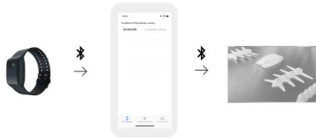
**Figure 1: E4 EDA Sensor (left), iOS app (middle), EDA Self-Interface (right). The E4 EDA sensor sends the participant data to the mobile app in real-time via Bluetooth. The mobile app processes the data and broadcasts select changes in the signal to the EDA Self-Interface via Bluetooth.**
