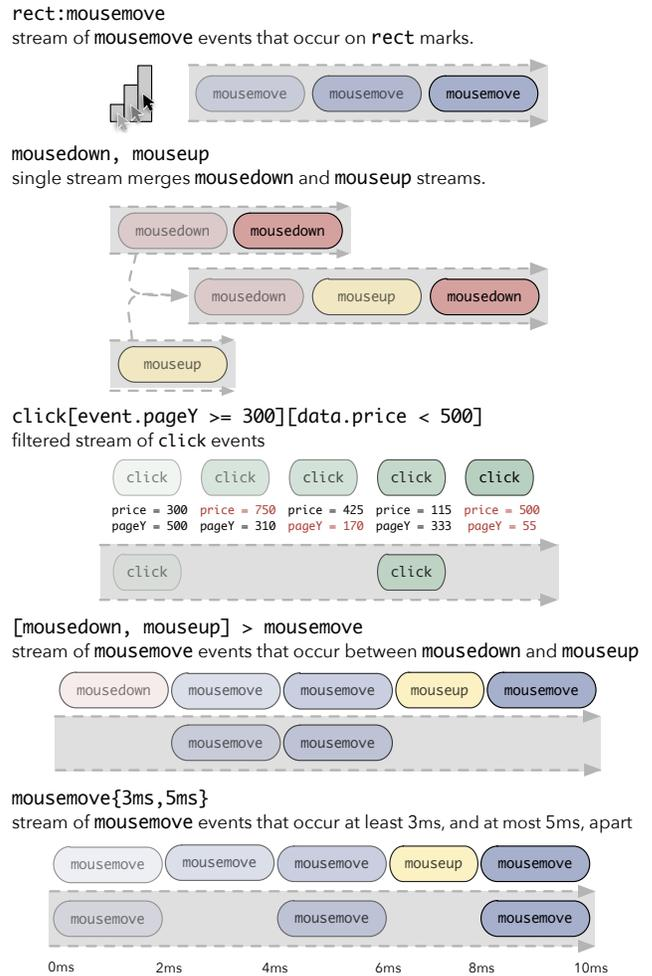
**Figure 2.** Event streams can be instantiated, composed, filtered, and sequenced using a syntax inspired by CSS3 selectors and regular expressions. This determines which events are captured by a particular stream (denoted by the dashed grey rectangles).
